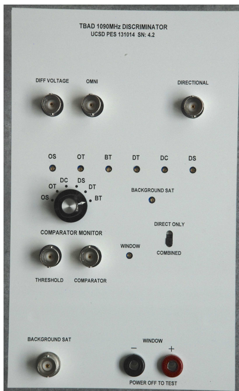
Figure 4: Discriminator box front, where threshold adjustments are made. The knob selects which threshold is made available to the THRESHOLD BNC, with trimpots labeled accordingly. Signals from the two RF power detectors are available, as is the differential amplifier (gain = 4) output. The various comparators associated with the six thresholds may also be monitored at the COMPARATOR connector, likewise knob-selectable. One may also adjust and monitor window width and background saturation duty cycle from the front panel. Finally, one may select whether transmitted DATA is based on directional signal (DT) alone, or combines omni (OT) as well.
