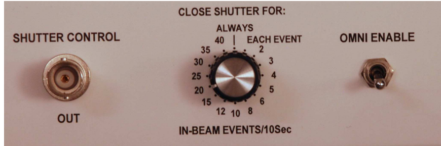
Figure 11: Decoder front panel controls, including the beam sensitivity adjustment and the OMNI enable switch. Here, the system is set for 20 events per 10 s, and the omni logging is disabled.
