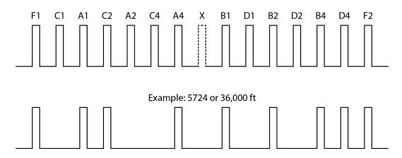
Figure 1: Mode-A/C pulse format. Pulses are 0.45  $\mu$ s in duration, separated by 1.45  $\mu$ s. The sequence is bracketed by framing pulses F1 and F2. The X format bit in the middle is not used in practice. The remaining 12 pulses define the 4-digit octal (ABCD) code.
